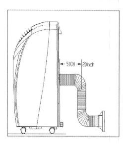
Incorrect Bending of the Exhaust can cause malfunction
